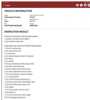
B. System Scan: automatically scan all systems of the vehicle
