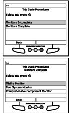
A "One moment please..." message displays while the Scan Tool retrieves the requested Drive Cycle Procedure. The Drive Cycle Procedures screen for the Monitor displays when the procedure has been retrieved.
