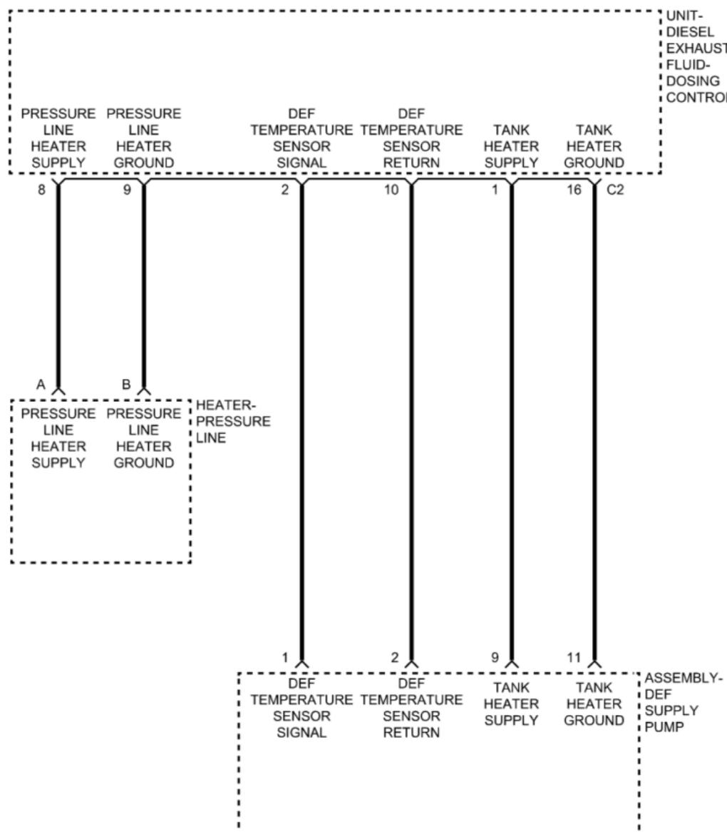
P202C wiring diagram
