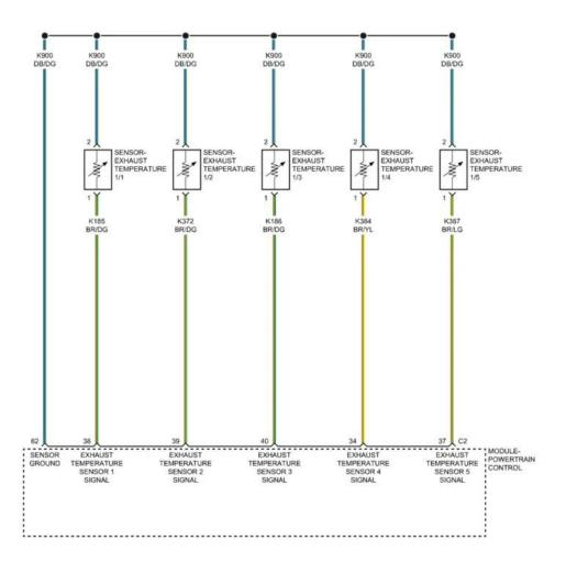
P200C wiring diagram
