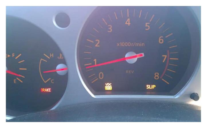
The VDC OFF and SLIP warning light turning on (Source: my350z.com)
